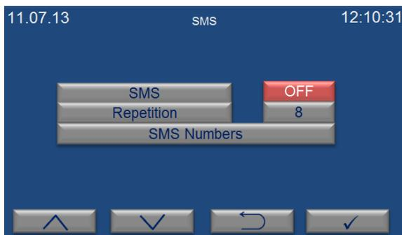
“SMS” submenu is selected on the menu page by the value increase (F1) and decrease (F2) keys. The page on the left appears when enter key (F4) is pushed. Submenus on SMS page is selected by using increase (F1) and decrease (F2) keys. Selected submenu can be adjusted by using enter key (F4). If you want to exit the page, push the backspace key (F3).
