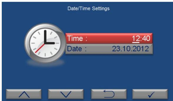
“Date/Time Settings” submenu is selected on the settings page by the value increase (F1) and decrease (F2) keys. The page shown on the left appears when enter key (F4) is pushed. Time is shown in the format of “hour:minute” and the cursor is on hour part when “Date/Time Settings” page comes to the screen. Hour is adjusted by pushing the value increase (F1) and decrease (F2) keys. Push enter key (F4) to
