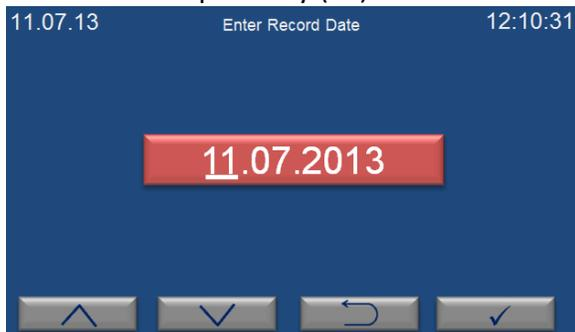
“History (TABLE)” submenu is selected on the memory page by the value increase (F1) and decrease (F2) keys. The page on the left appears when enter key (F4) is pushed. Enter a date to analyze corresponding operation by pushing the value increase and decrease keys. Push the enter key (F4) to access the table.
