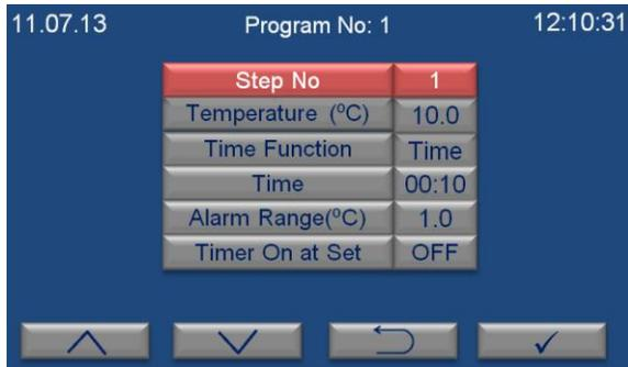
The step settings screen on the left appears, when enter key (F4) is pushed when the selection is on program on the operations settings screen.
