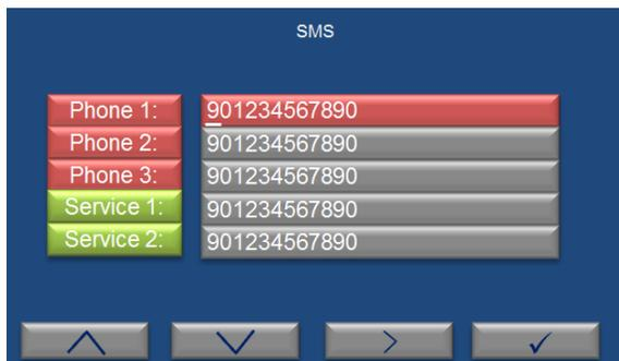
“SMS Numbers” is selected on the SMS page by using the value increase (F1) and decrease (F2) keys. The page on the left appears when enter key (F4) is pushed. The phone numbers can be entered in this page and SMS notifications are delivered to these phone numbers in case of any failure.
